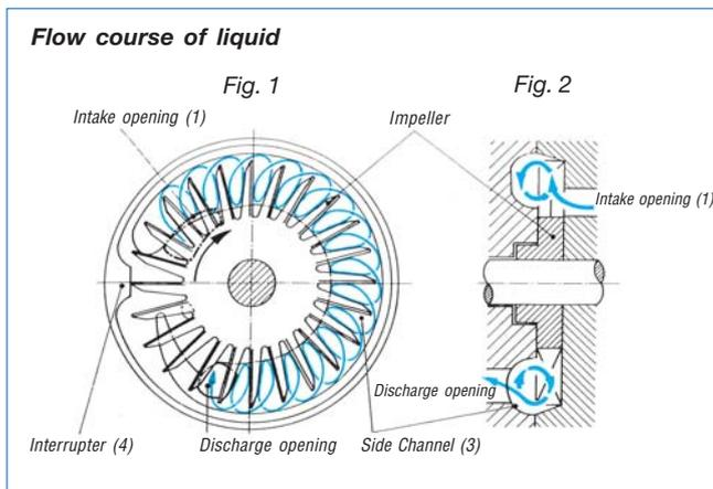
The centrifugal effect of the impeller separates air from the liquid. The liquid collects in the outer region of the impeller cells and side channel, whereas the air builds up in the inner part (5).
