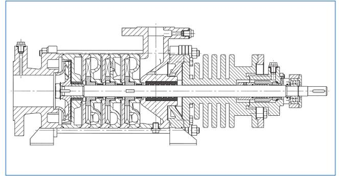
When mounting the centrifugal impellers, either one or two, in a series connection with one or more Side Channel Stages, the specific favorable characteristics of the two delivery principles complement one another.
